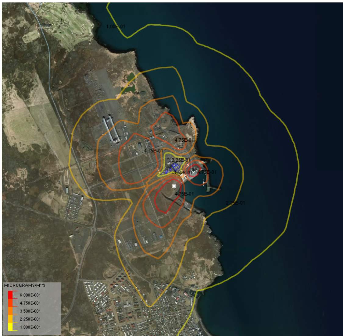
Figure 19. Discharge through a hypothetical emergency stack assuming the oven runs 15MW . The concentrations plotted represent annual maximum value. Emission details are provided in Table 2.
