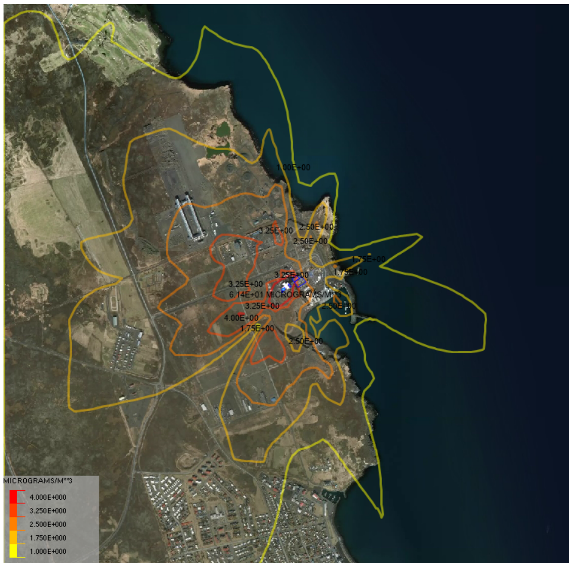
Figure 7. Discharge through filter bag house rooftop assuming the oven running on 10MW. The concentrations plotted represent annual maximum value. Emission details are provided in Table 2.
