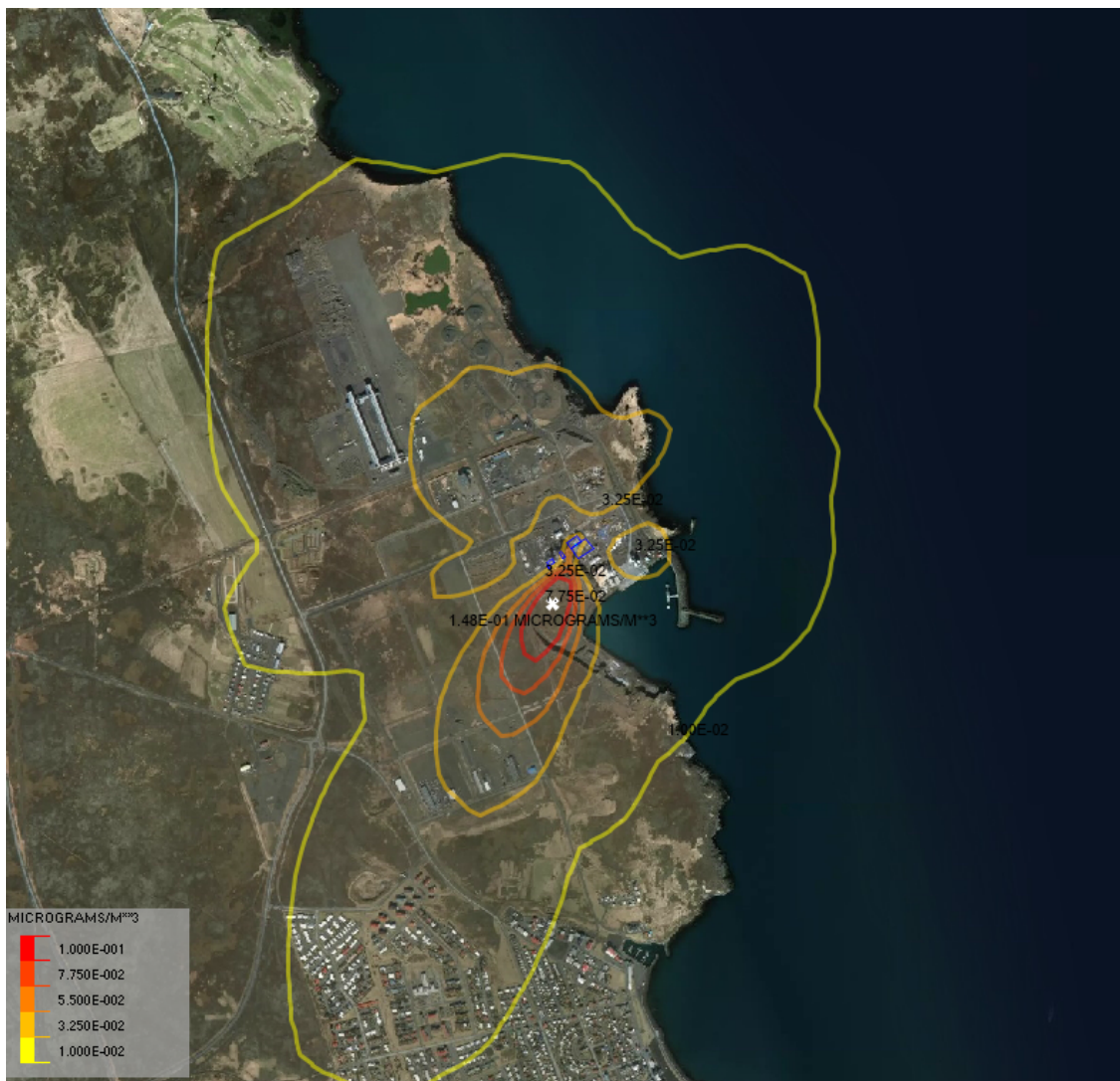
Figure 26. Discharge through a hypothetical emergency stack assuming the oven was shut down 6 hr ago. The concentrations plotted represent annual average value. Emission details are provided in Table 2.
