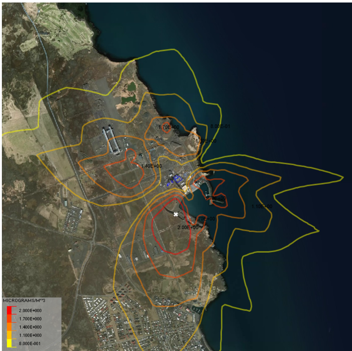
Figure 25. Discharge through a hypothetical emergency stack assuming the oven was shut down 6 hr ago. The concentrations plotted represent annual maximum value. Emission details are provided in Table 2.
