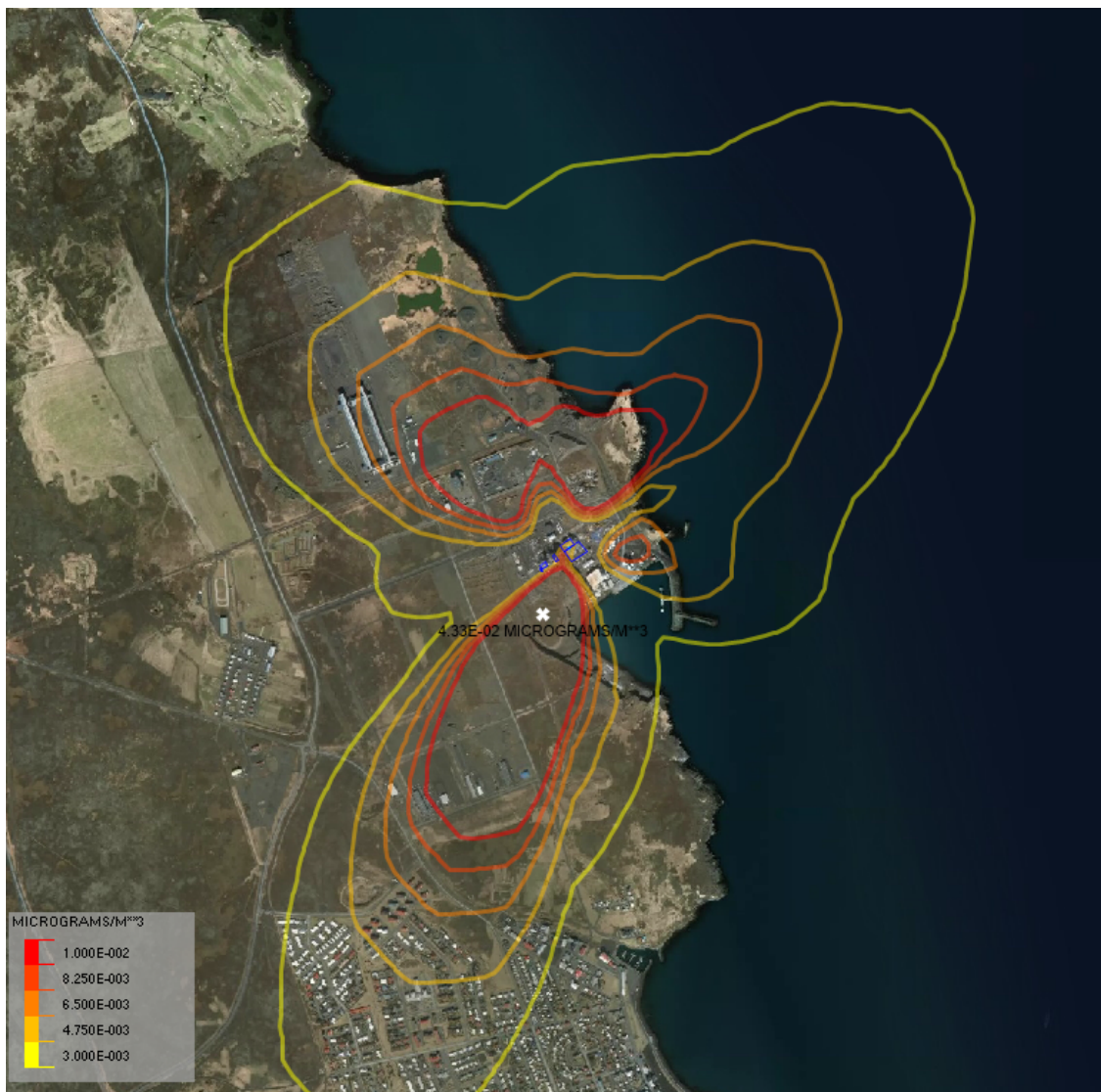
Figure 20. Discharge through a hypothetical emergency stack assuming the oven runs 15MW . The concentrations plotted represent annual average value. Emission details are provided in Table 2.
