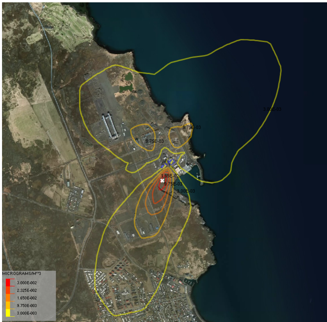
Figure 18. Discharge through a hypothetical emergency stack assuming the oven runs 20MW . The concentrations plotted represent annual average value. Emission details are provided in Table 2.
