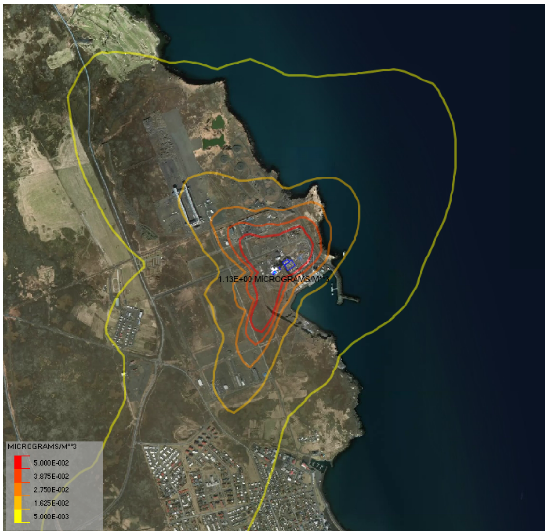
Figure 6. Discharge through filter bag house rooftop assuming the oven running on 32MW. The concentrations plotted represent annual average value. Emission details are provided in Table 2.
