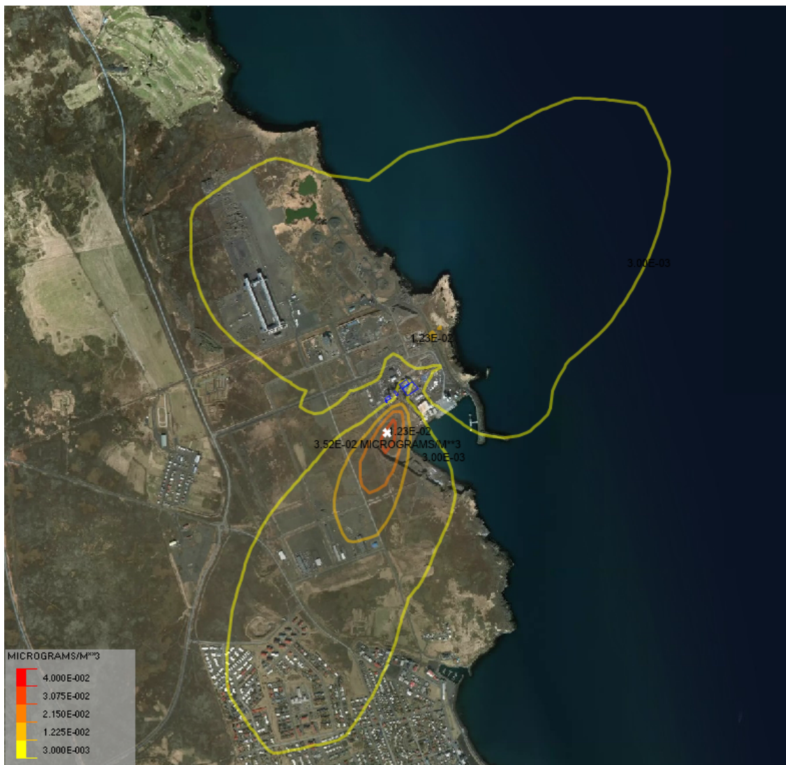
Figure 16. Discharge through a hypothetical emergency stack assuming the oven runs 32MW . The concentrations plotted represent annual average value. Emission details are provided in Table 2.
