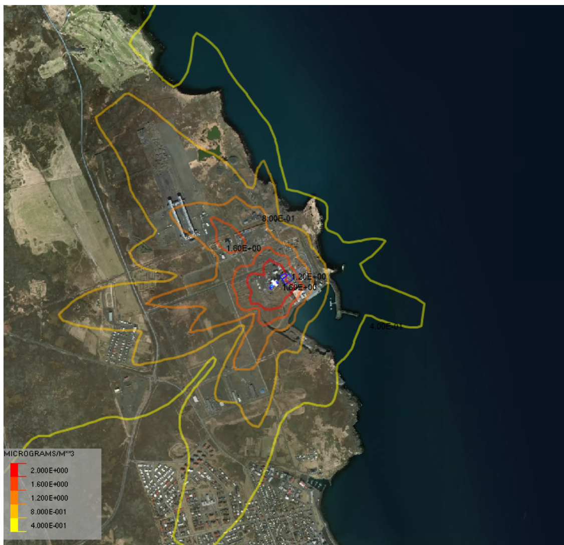
Figure 5. Discharge through filter bag house rooftop assuming the oven running on 32MW. The concentrations plotted represent annual maximum value. Emission details are provided in Table 2.
