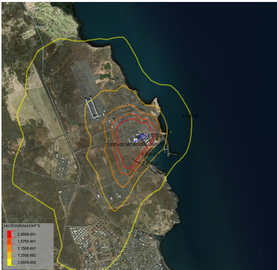
Figure 14. Discharge through filter bag house rooftop assuming the oven was shut down 1.5 hr ago. The concentrations plotted represent annual average value. Emission details are provided in Table 2.
