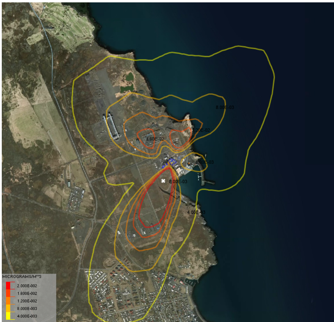
Figure 22. Discharge through a hypothetical emergency stack assuming the oven runs 10MW . The concentrations plotted represent annual average value. Emission details are provided in Table 2.
