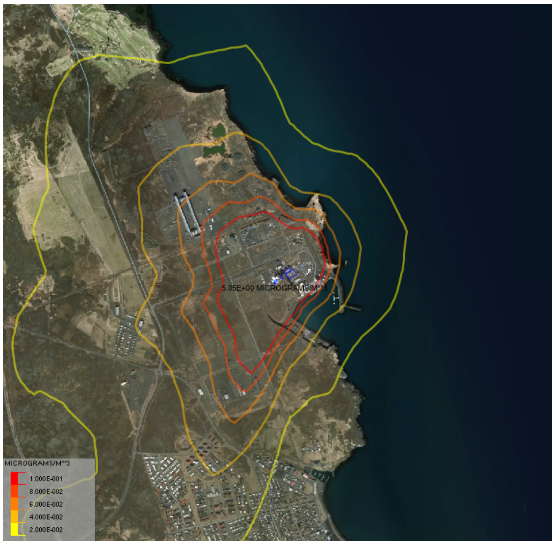
Figure 12. Discharge through filter bag house rooftop assuming the oven was shut down 1 hr ago. The concentrations plotted represent annual average value. Emission details are provided in Table 2.
