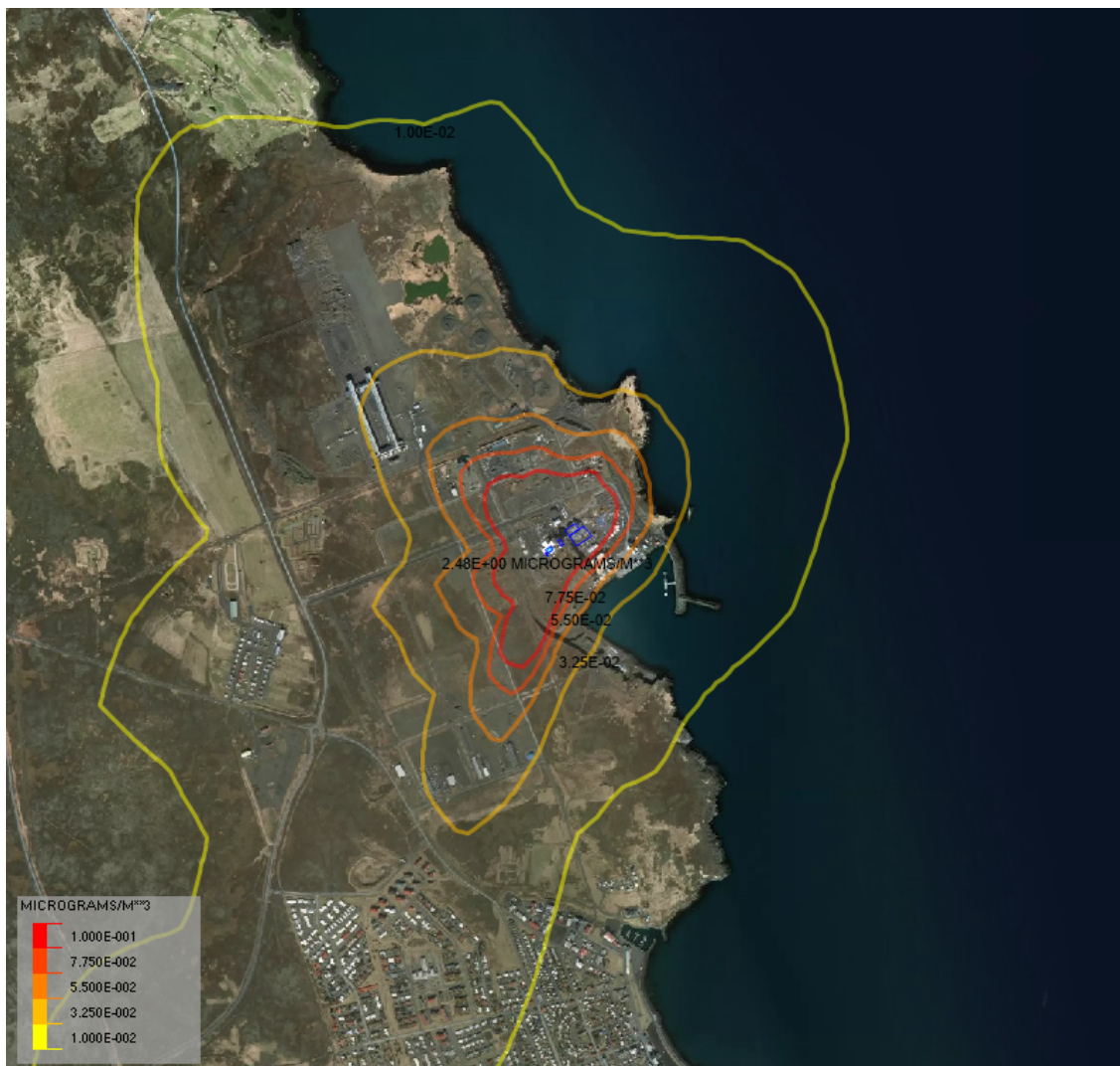
Figure 8. Discharge through filter bag house rooftop assuming the oven running on 10MW. The concentrations plotted represent annual average value. Emission details are provided in Table 2.
