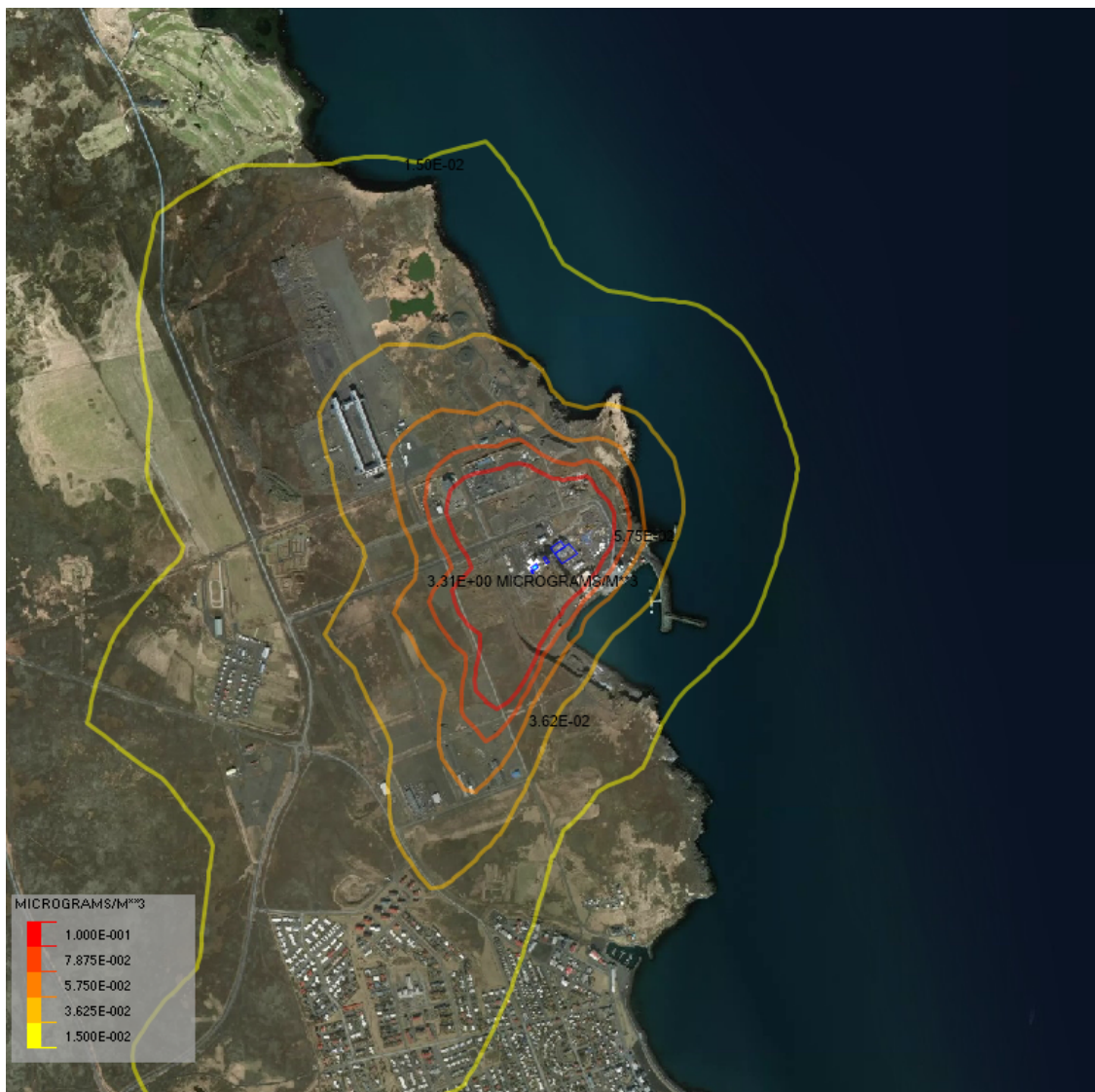
Figure 10. Discharge through filter bag house rooftop assuming the oven was shut down 0.5 hr ago. The concentrations plotted represent annual average value. Emission details are provided in Table 2.
