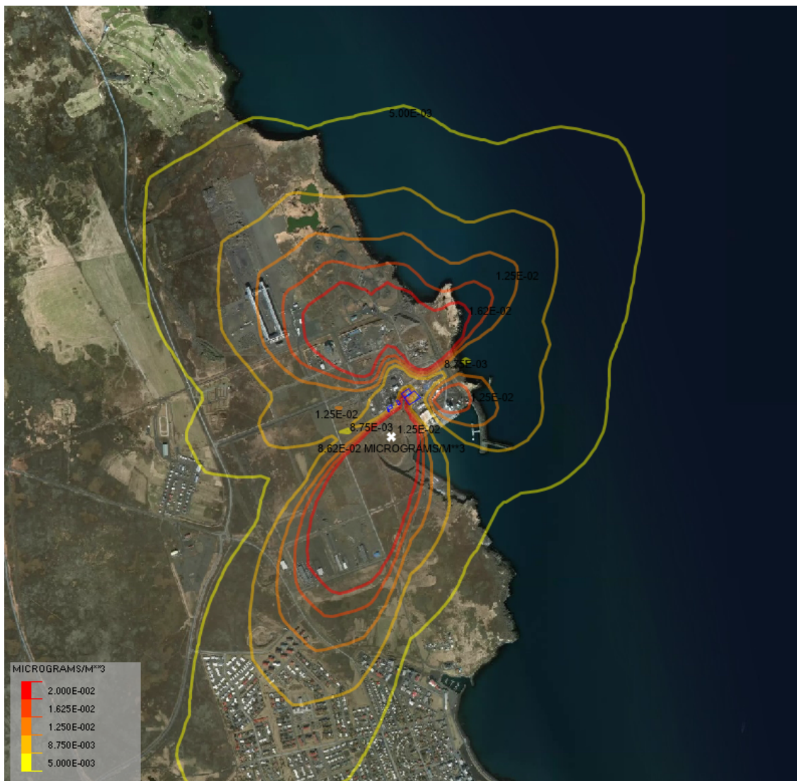
Figure 24. Discharge through a hypothetical emergency stack assuming the oven was shut down 3 hr ago. The concentrations plotted represent annual average value. Emission details are provided in Table 2.
